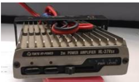
Tokyo 144MHz Power Amp (28) Built in RX Preamp 3W in 30W Out £20
