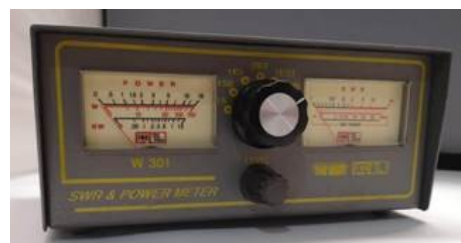
W-301 SWR & Power Meter (5) 30MHz 1.5KW £15
