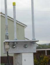
(Note: When cutting the threads, make sure they are perfectly square, else you will end up with an antenna that looks a bit strange with elements leaning at odd angles. Also, aluminium will tend to grab the tap or die so a little lubricant will help give you a clean thread, but make sure you clean it thoroughly before final assembly.)
